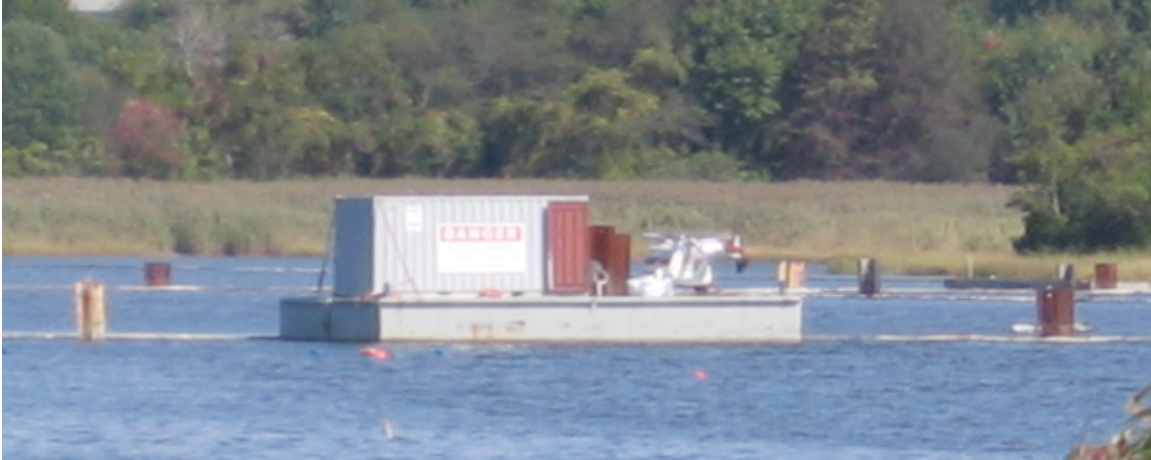
The dredge is towed by cables from the shore
