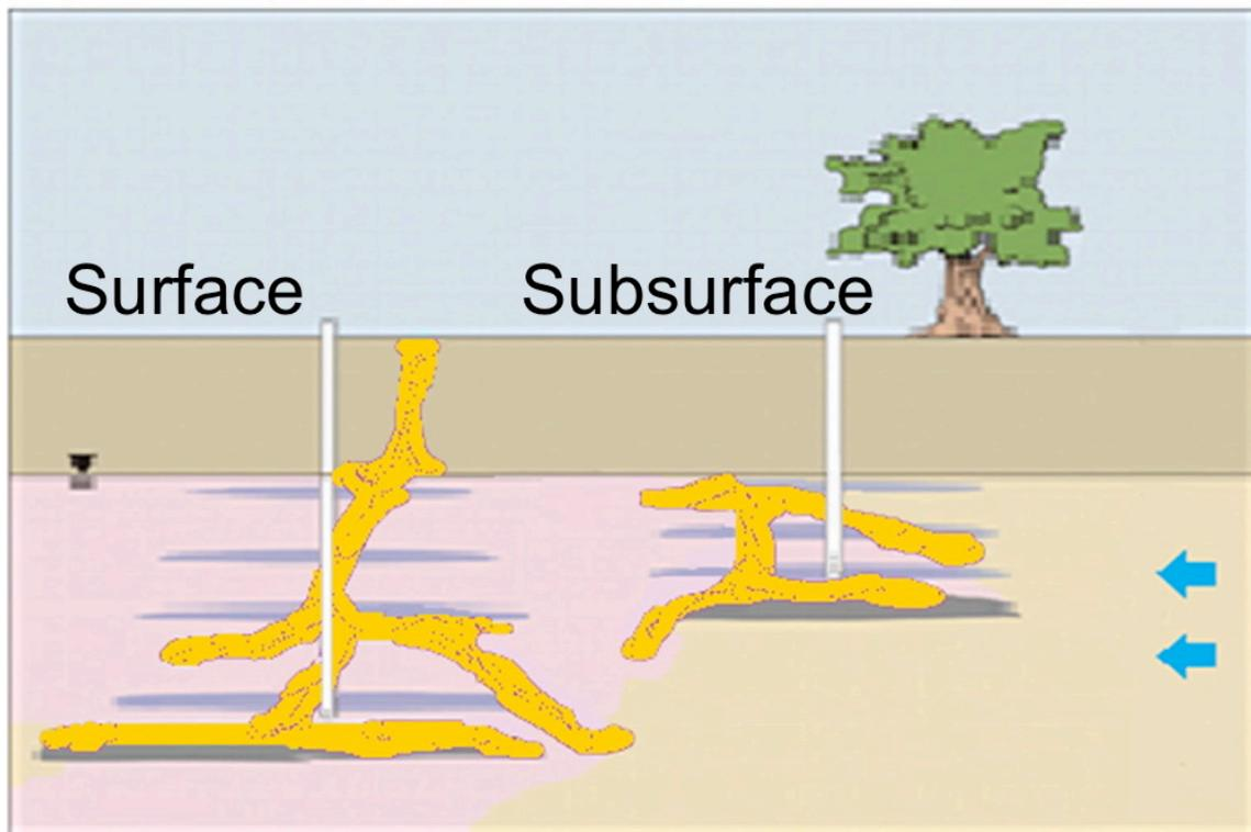
**EPA diagram showing the difference between contamination released at the surface and contamination from a subsurface pathway. The vertical bars represent monitoring wells.**
